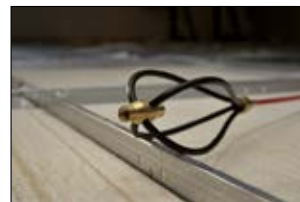
The whisk allows the rod to glide over obstructions easily.
